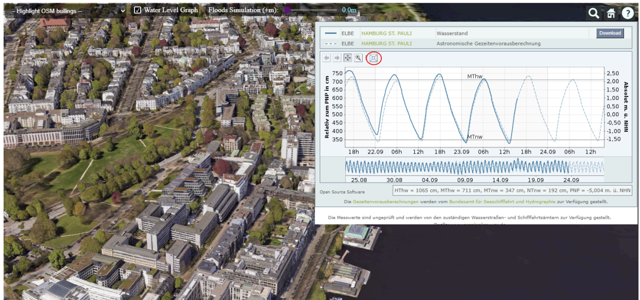
Fig. 11: Water level diagram of the St. Pauli measuring station
