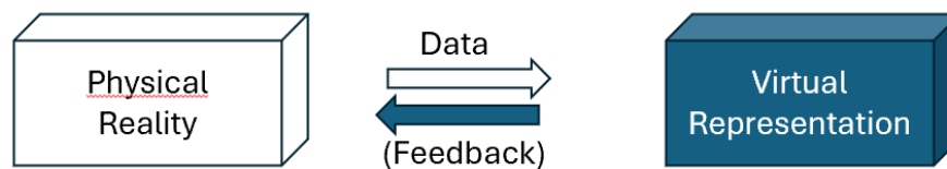
Fig. 2: Components of a Digital Twin and their relationship
