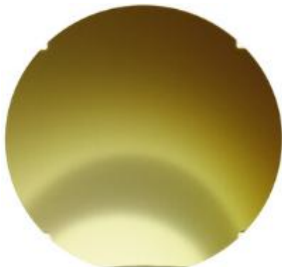
1) Piotrowiak et al. : Continuous materials library of La-Co-Mn-Fe on a single crystal \text{Al}_2\text{O}_3 -substrate (with a 100 mm diameter)
