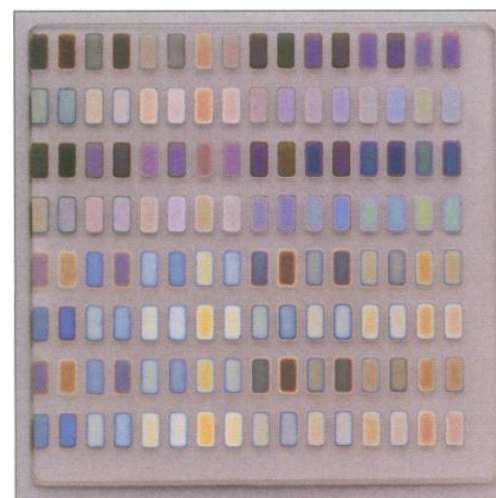
2) Xiang et al. : Discrete materials library of with MgO single crystal as substrate (each discrete site is 1x2 mm)
