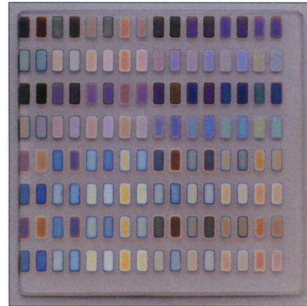
Fig. 3. A 128-member binary library prior to sintering. Each site is 1 mm by 2 mm; the color of each is the natural color of reflected light from a white light source. The library was deposited according to the sequence 1, Bi, M0 (no secondary mask); 2, Bi, M1; 3, Cu, M0; 4, Cu, M2; 5, Cu, M3; 6, Sr, M0; 7, Sr, M5; 8, Ca, M6; 9, Cu, M4; 10, Ca, M7 (9). The molar stoichiometry for each layer was 1:1 relative to Bi (which was deposited as a 300 Å layer), with the exception of steps 3 and 5 in which the Cu:Bi ratio was 0.5:1.
