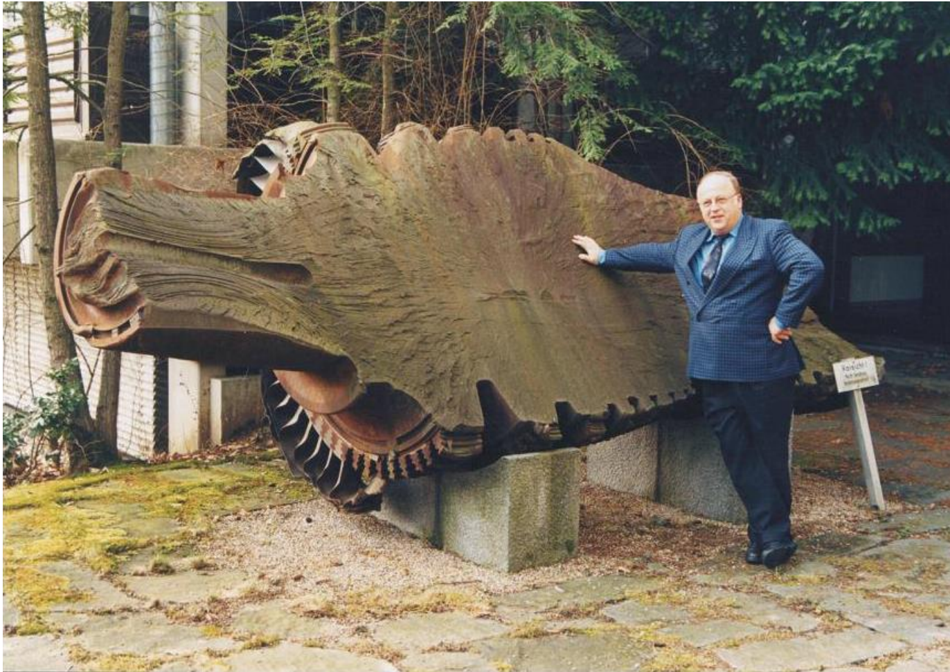
Piece 26 of turbine rotor which failed in 1987 (Power Plant Irsching). Failure analyst Prof. M. Pohl (IFM-RUB) at Allianz Zentrum für Technik (AZT) in Ismaning, Februar 2000.
