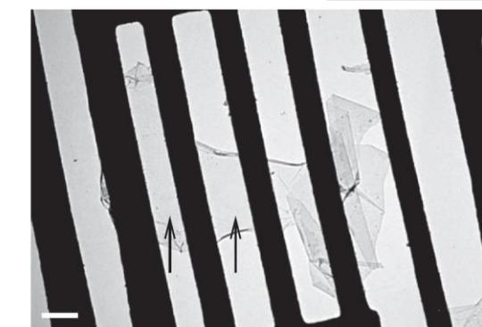
Figure 1 | Suspended graphene membrane. Bright-field TEM image of a suspended graphene membrane. Its central part (homogeneous and featureless region indicated by arrows) is monolayer graphene. Electron diffraction images from different areas of the flake show that it is a single crystal without domains. We note scrolled top and bottom edges and a strongly folded region on the right. Scale bar,  $500$  nm.
