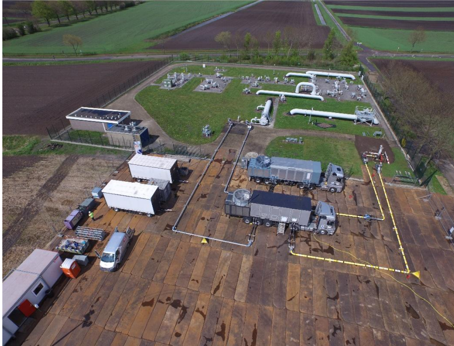
Mobile compressor (Source: Open Grid Europe, 2020)
