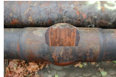
Knuckle Joints for Protection of Old Joints
