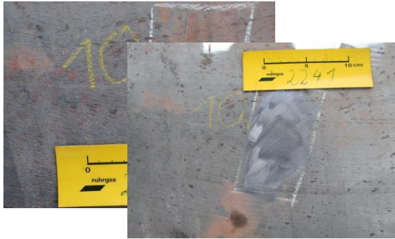
Smooth Grinding of Corrosion or Gouge
