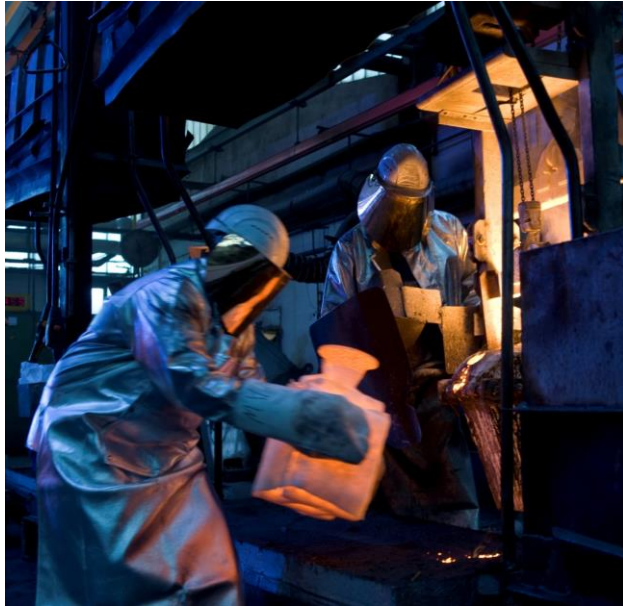
Burn-out and pre-heating the shell
