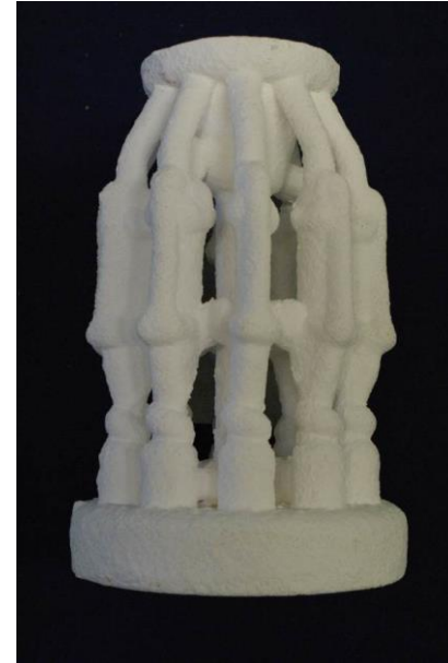
Slurry dipping and coating
