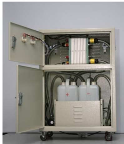
Vanadium Redox Flow Battery, Shanefelan https://www.flickr.com/photos/shanephelan/3704404831/
