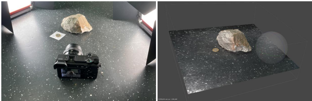
Figure 2. Image recordings of samples collected in the field. Left: photo of image recording's setup. Right: digital 3D-model in Agisoft Metashape.
