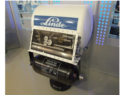
Tank for liquid H 2 compared against a high pressure H 2 cylinder below, Museum Autovision, Altlußheim, Germany (Author= Claus Ableiter)
