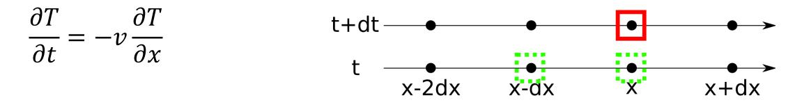
$$\frac{T_x^{t+dt} - T_x^t}{dt} = -\nu \frac{T_x^t - T_{x-dx}^t}{dx}$$
