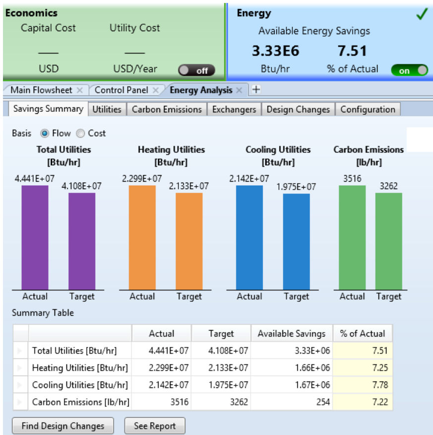
Figure 16.29 The energy analysis results shown in different forms and the potential savings.
